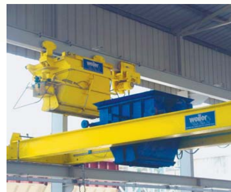
Automated concrete shuttle
